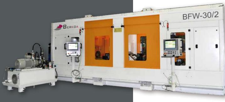
► Friction spin welding machine with two stations.
