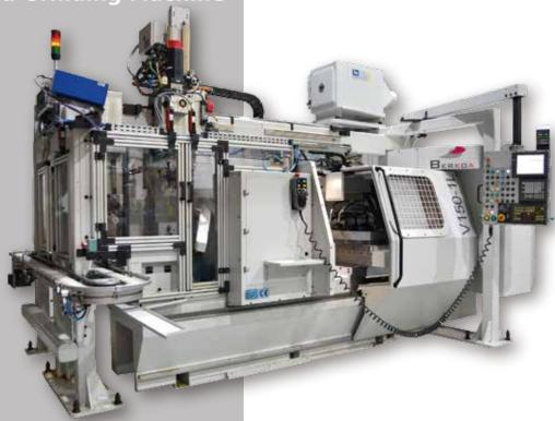
$^{ullet}$  Production Machine for Inner Grinding of Cams.
